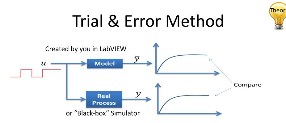
Adjust model parameters and then compare the response from the real system with the simulated model. If they are "equal", you have probably found a good model (at least in that working area)
