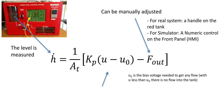
We need to find the unknown model parameter(s) using System Identification methods
